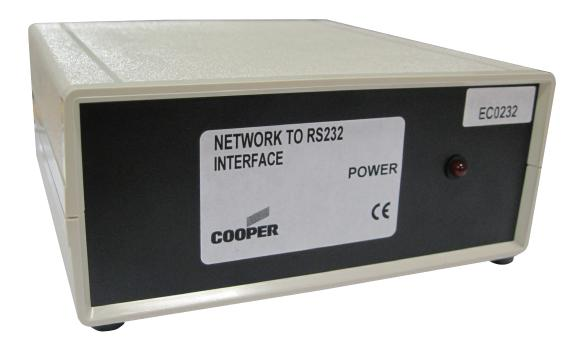
The (EC0232) Lon to RS232 adapter allows connection of the Cooper system network (LonWorks) devices to PC based applications such as site monitor, site graphics.
