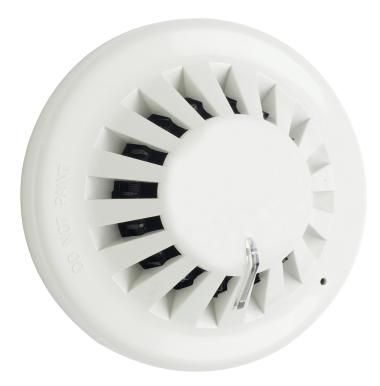
The conventional range offers a multi-mode, 5 in 1 detector (FXN922), covering many building needs. It's quick and simple to install with a stylish low profile design. The detector is mounted on our standard conventional base (FXN520) but can also be used in conjunction with our relay base (FXN520R) for local switching. Each detector is fitted with a 360° viewable LED for indication.
