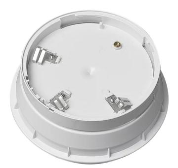
The KAC DB sounder is a high quality 32 tone sounder featuring fast and simple installation and control and forms the perfect base for SS detectors. It is powered by the fire panel via the loop wiring. Control of the device is enabled using on-board switches some of which can also be adjusted through SS Advanced Protocol.
